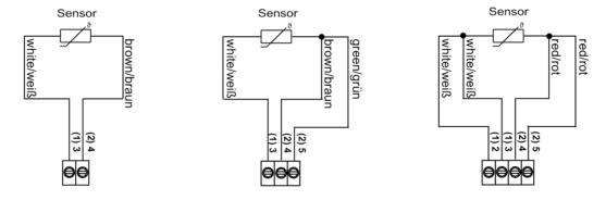
fig. (terminal assignment passive sensor)
