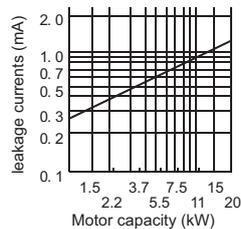
For "Δ" connection, the amount of leakage current is approx. 1/3 of the above value.
