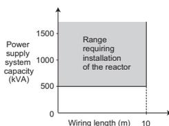
To prevent this, always install an optional AC reactor (FR-HAL). When connecting a single-phase 100V power input model to a power transformer (50kVA or more), install an AC reactor (FR-HAL) so that the performance is more reliable.
